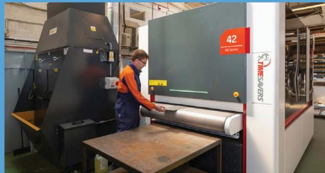
Dutton Engineering make good use of a Timesavers' 42 series machine for both deburr and grinding operations in a single pass
