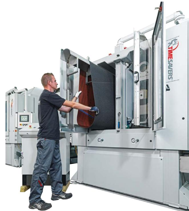
All Timesavers' machines are designed for ease of maintenance. Replacing grinding belts (here shown on an 81 series machine) is much more straightforward compared to a grinding stone.
