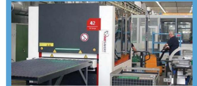
Krones' machine park is equipped with a WRB42 series rotary brush machine which enables deburring and final edge rounding in a very efficient one-step operation
