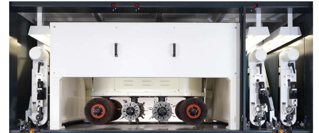
The extremely versatile 42 series can be specified with various carousel rotating brush heads and grinding belts for or flawless deburring, perfect edge rounding, high-class finishing and ultimate precision grinding
